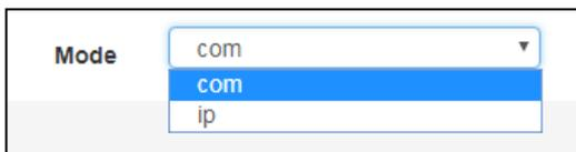
To use a serial connected GSM modem, select com as operating mode..
