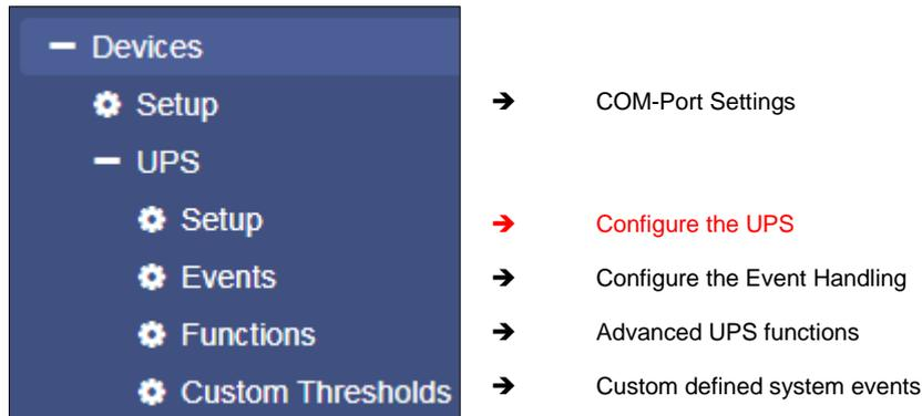
After configuring COM1 to use UPS, go to the submenu UPS and forward to Setup:
