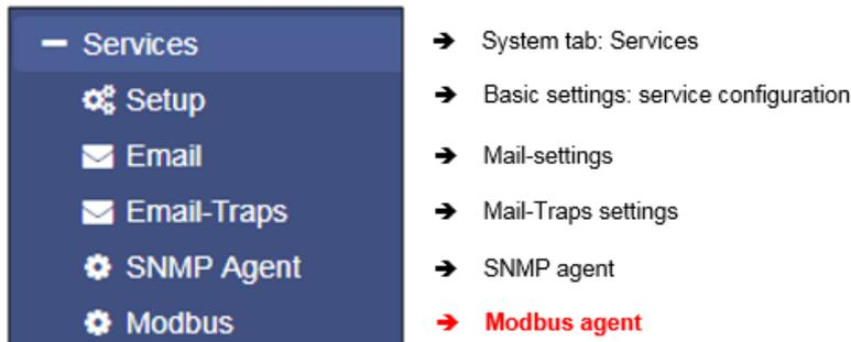
Since Modbus is standardized, the basic configuration is intuitive to handle. To configure the modbus agent, go to services and open Modbus.
