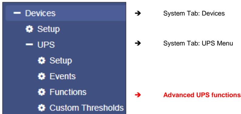
The UPS Functions menu contains options to perform tests sequences or to configure build-in special functions a UPS may provide. They are tailored to the UPS model used to represent its functionality. As a consequence, the functions displayed for this menu item can vary - some UPSs only allow the on / off state as well as a single test-button, others provide more functionality.
