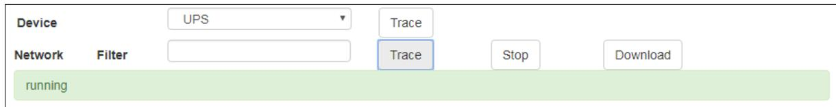
The Tracer logs packet data within the LAN segment in real-time and stores it locally on the CS141. The tracer will quit if there are two conditions:
