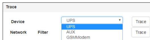
The Tracer is a comprehensive diagnostic tool for verifying communication between the CS141 and the connected devices as well as for identifying network problems.
