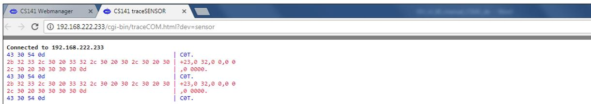
The trace ends automatically by closing this tab. Please note that the data will be discarded. To save the data, mark it with the left mouse button and copy the content with CTRL + C, and insert the information with CTRL + V to a text file.
