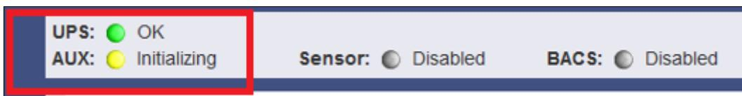
The UPS is set correctly and has made the communication accordingly. The AUX port, on the other hand, is set to initializing. However, since the AUX port has no device connected to CS141, the yellow marker will change from yellow to blue in time, while the LEDs on the front of the CS141 continue to glow green and red statically.
